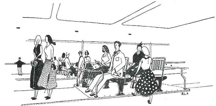
Articulated platforms move continuously around the building in opposite directions. Seats are placed at intervals, and from these can be seen views of the industrial Black Country, the shop windows, and occasionally the central area of the building. As these platforms move very slowly it is quite easy to walk over them to reach the six glazed observation terraces over the entrance.
